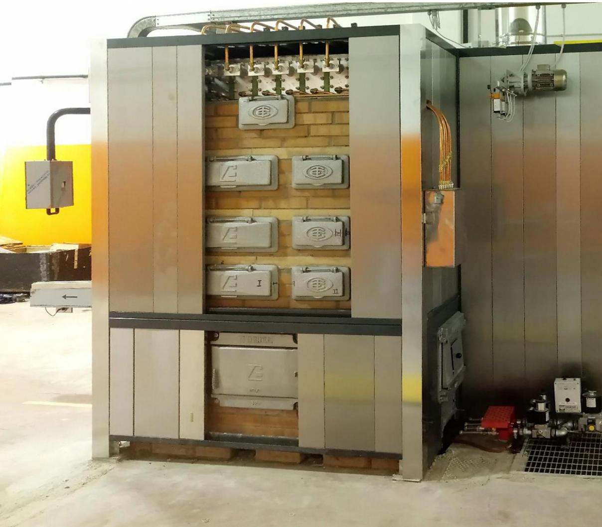
This is the heart of the system. The combustion chamber is made of refractory bricks, carefully laid from our specialized technicians with specific volumes and angles in order to drive the heat precisely to each group of pipes for perfect heat distribution in the baking chamber. It is designed for Very long life expectancy.
