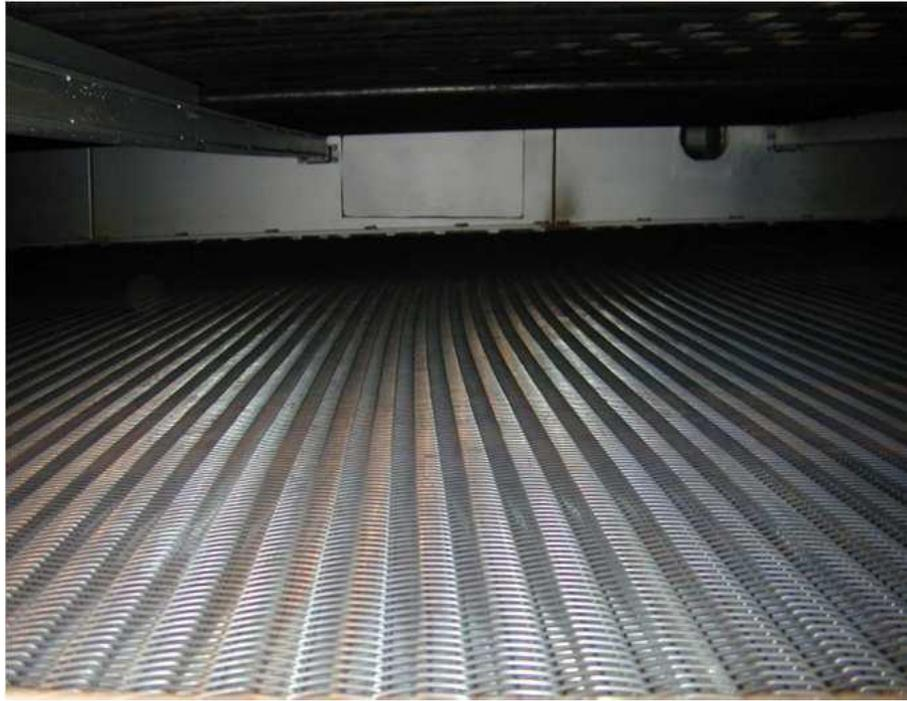
Stone belt is ideal for crusty/ rustic bread that requires baking directly onto the stone hearth
