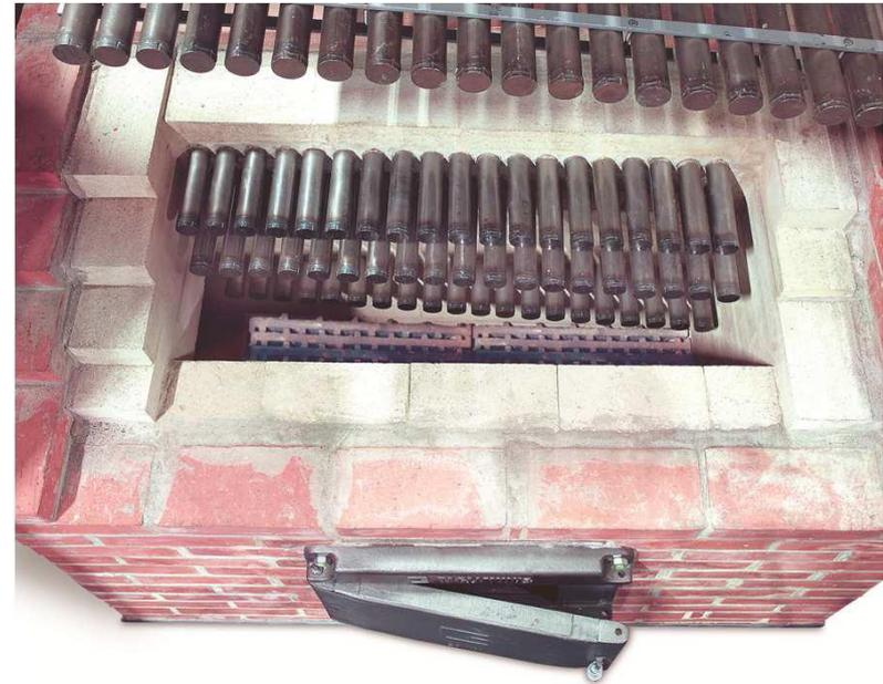
**Every pipe is filled with water and closed individually, with a special technique called «friction welding». Because of this, the pipe sealing becomes unbreakable.**
