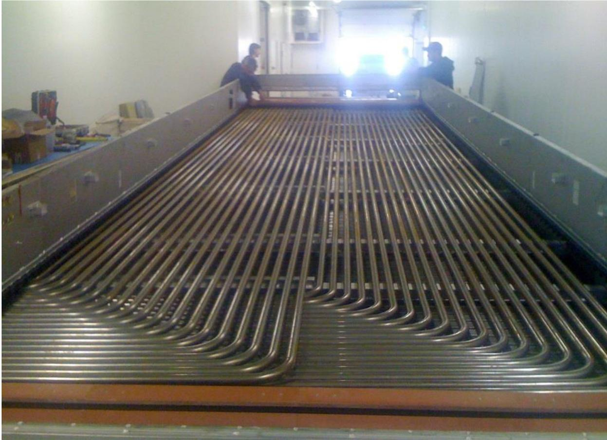
**Each pipe is sealed at both ends and contains a precise amount of distilled water according to the length of the pipe.**
