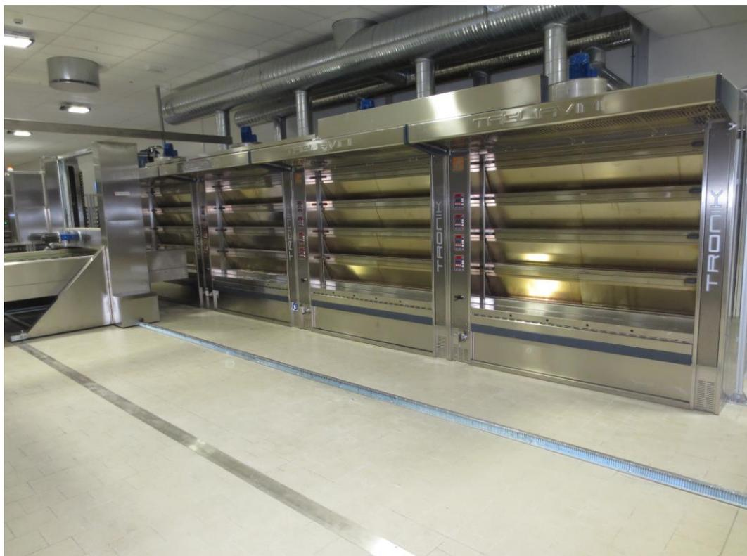
n.4 Tronik deck ovens served by a Robot Loader, with boards pre loading and automatic unloading on accumulation belt
