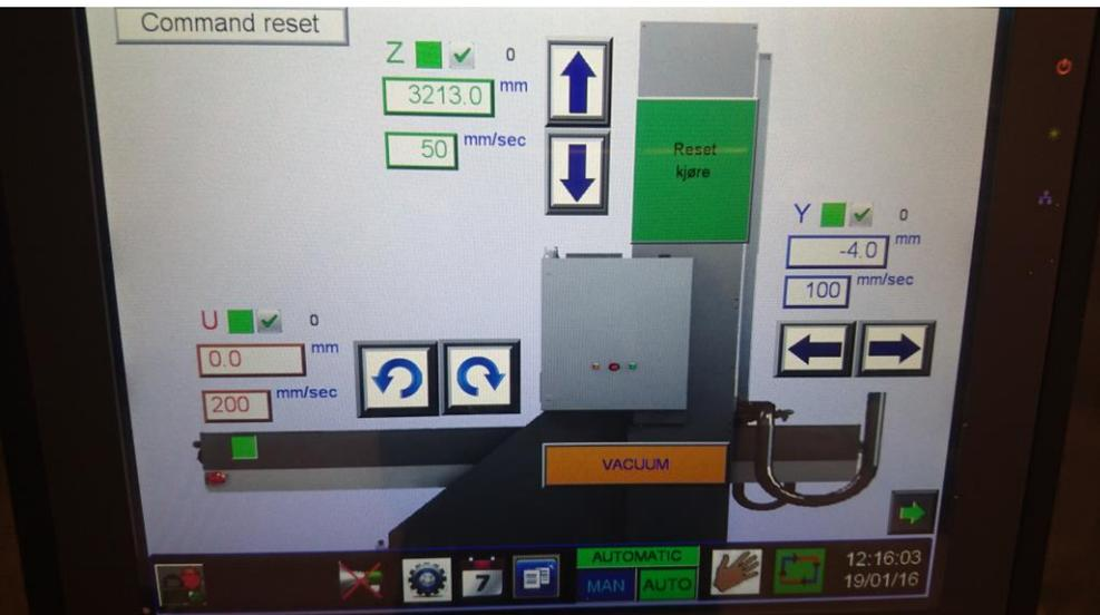
Touch screen PLC to control all phases of the process
