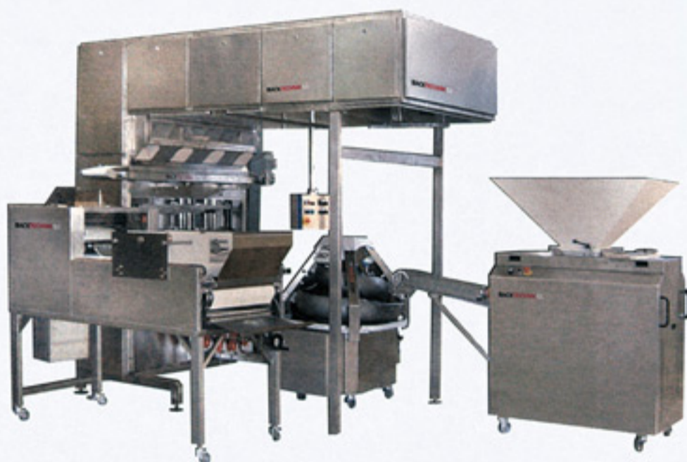
The CPL bread line features a Soft 3B dough divider, an Allround conical rounder, a Timer intermediate proofer and a Max long moulder
