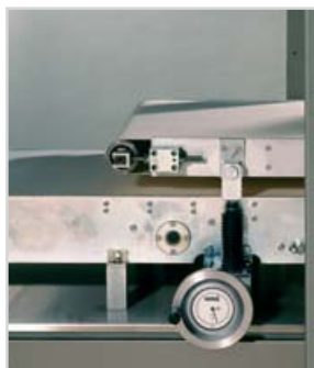
Long-moulding unit with movable top belt
