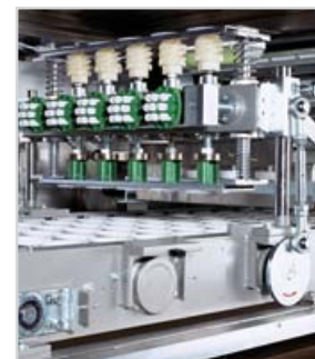
Forming unit inside the Vario-Star
