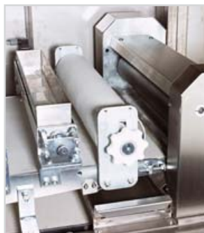
Sheeding head Long-moulding unit with fixed pressure board:
