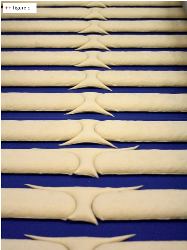
++ figure 1 21 varieties of baguette and petit pain products are stamped out of the respective dough sheets on the production line
